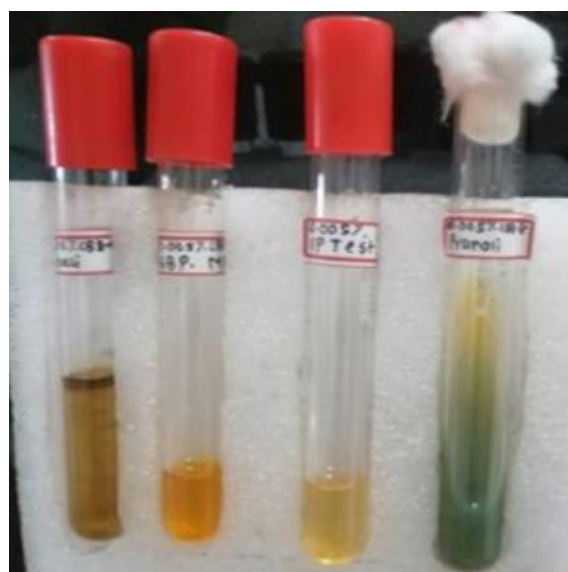
Fig 4: IMViC test for identification of isolates obtained on plate with 0.005% Coomassie brilliant blue-G.
