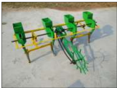
Fig 1: ICAR-NRRI urea briquette applicator
