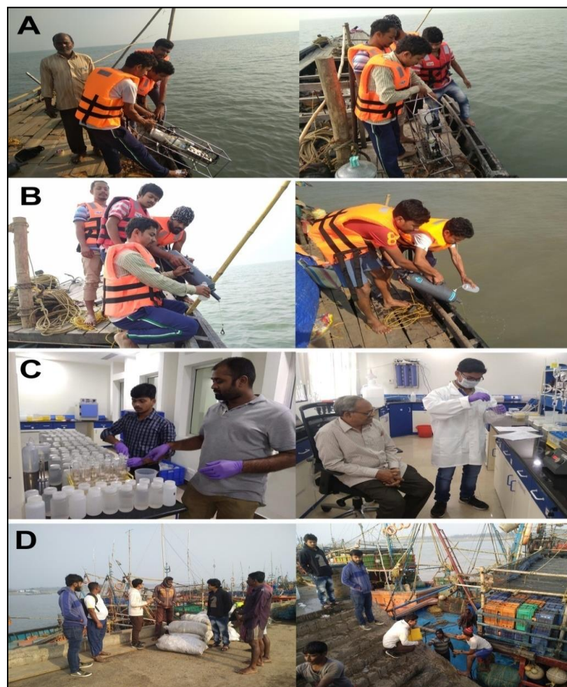
Fig 8: (A) In-situ water quality measurement through CTD; (B) Water sample collected for chemical analysis through Niskin Sampler; (C) Chemical analysis of water sample in the Laboratory and (D) Respondent survey with the fisherman for collecting the fish catch data.
