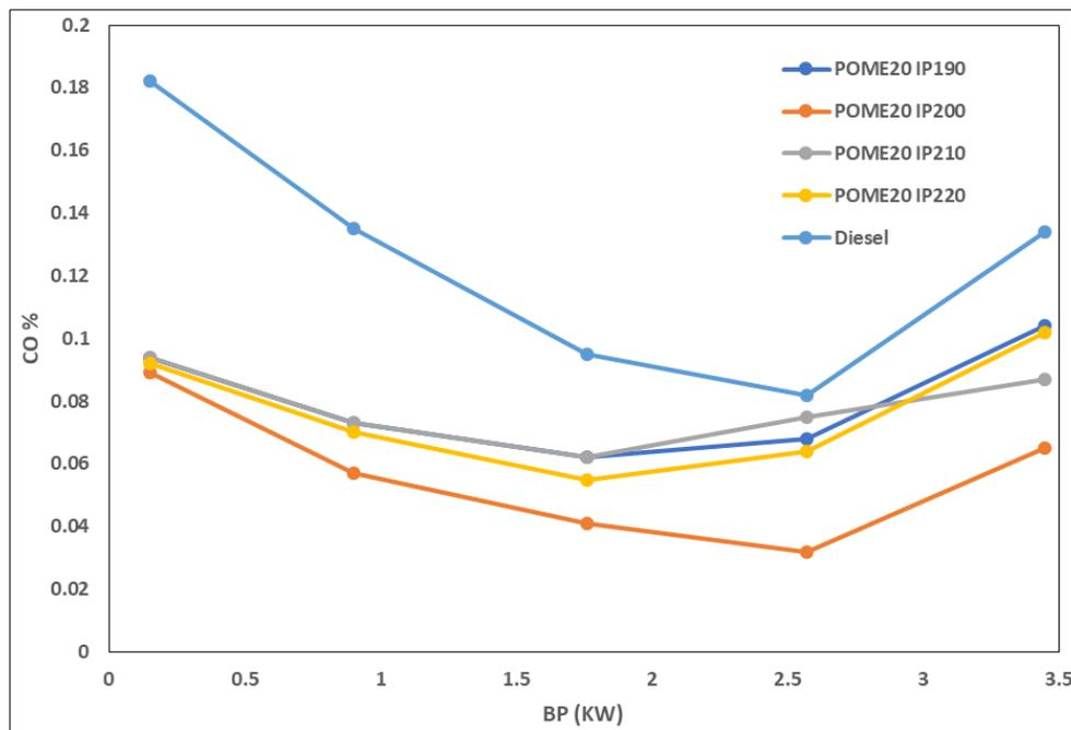
Fig 10: Impact of Injection Pressure on Carbon Monoxide emissions
