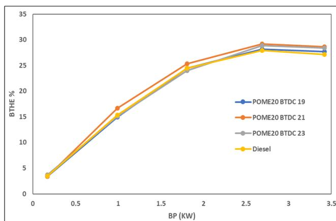
Fig 11: Impact of Fuel Injection time on Break Thermal Efficiency
