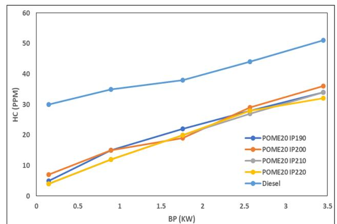
Fig 9: Impact of Injection Pressure on Unburnt Hydro carbons
