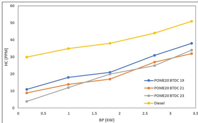
**Fig 13:** Impact of Fuel Injection time on Emissions of Unburnt Hydro Carbons
