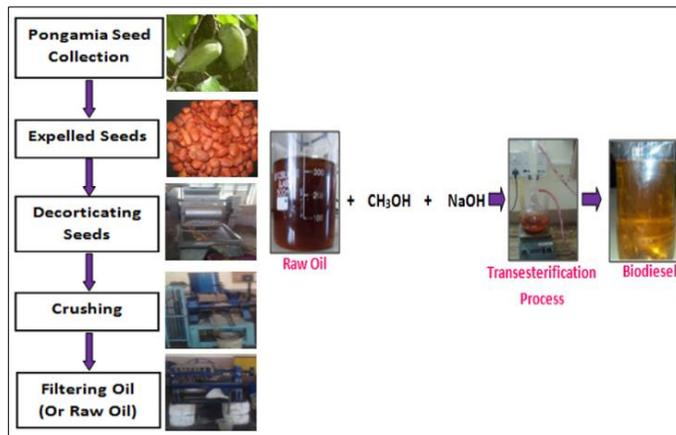
**Fig 1:** Pongamia Biodiesel Preparation
