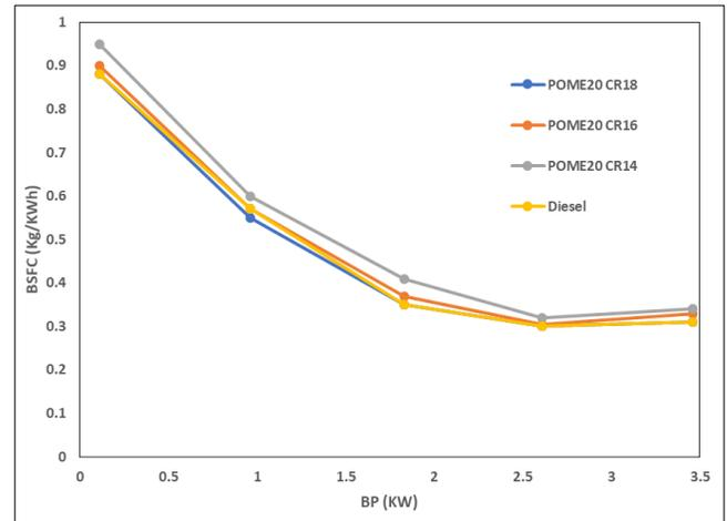
**Fig 4:** Impact of Compression ratio on BSFC
