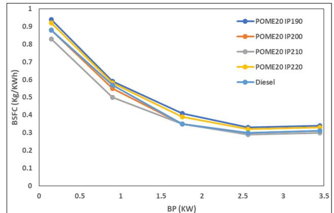
Fig 8: Impact of Injection Pressure on BSFC
