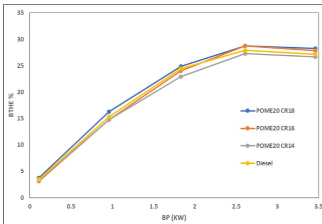
**Fig 3:** Impact of Compression ratio on Break Thermal Efficiency
