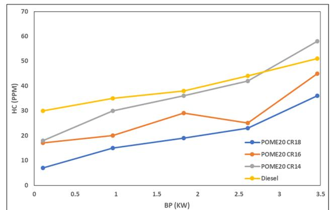
**Fig 5:** Impact of Compression ratio on Unburnt Hydrocarbons
