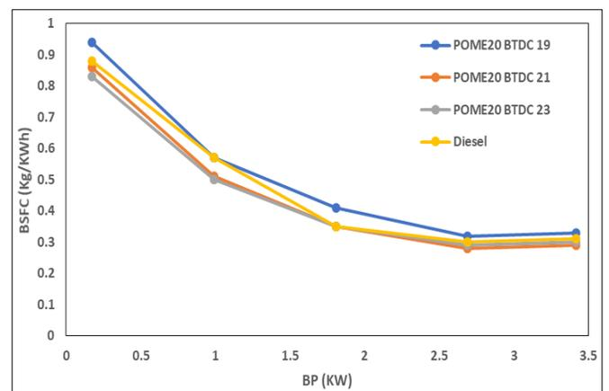
Fig 12: Impact of Fuel Injection time on BSFC
