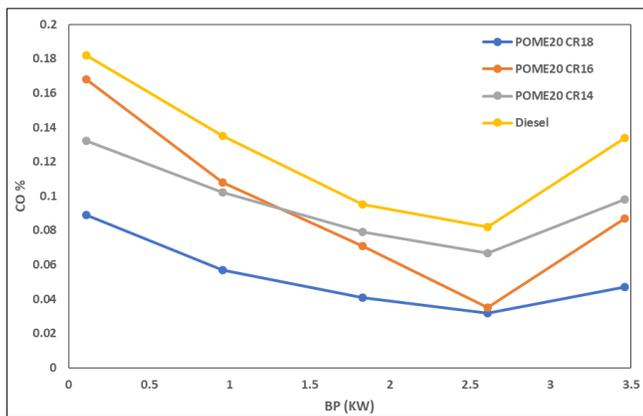
Fig 1: Impact of Compression ratio on Carbon Monoxide
