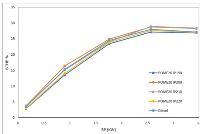
Fig 7: Impact of Injection Pressure on Break Thermal Efficiency
